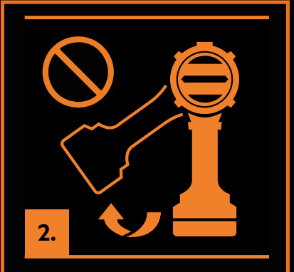
2. ANTI-KICKBACK technology engages & prevents the tool from over-turning
